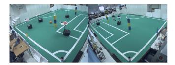
Figure B.1: Snapshot from the GTS installed for ground truth evaluation of the ball's 3D positions and the robots' 2D positions.
