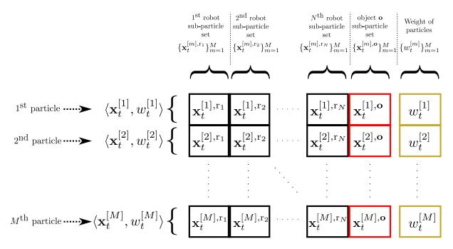
Figure 5.4: Tabular representation of the particles, sub-particles and the associated notations defined in Section 5.4 and used in Algorithm 5.1 and subsequently.
