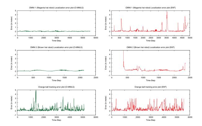
Figure 5.2: 2 robots experiment: The X-axis in these plots represent the number of time-steps between two consecutive GTS frames. If for a particular robot or the ball the GTS could not estimate the GT, error w.r.t. it is not computed at that time step and hence omitted from the plots. The Y-axis represents the position error which is the Euclidean distance between the GT position estimates and the O-MMLG (left) or EKF (right) estimates of the robot and the orange ball positions.
