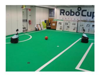
Figure 4.5: Real robot view for one of the layout locations: the robot on the left is the robot that informs the correct ball position to the other, while the robot on the right is the kidnapped robot which uses that information, in location 4 of Figure 4.4.
