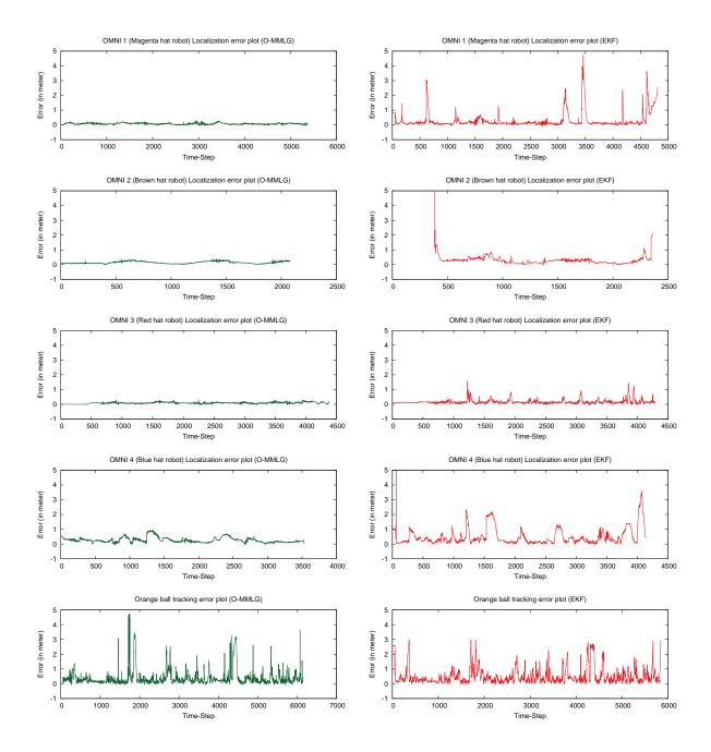
Figure 5.3: 4 robots experiment: The X-axis in these plots represent the number of time-steps between two consecutive GTS frames. If for a particular robot or the ball the GTS could not estimate the GT, error w.r.t. it is not computed at that time step and hence omitted from the plots. The Y-axis represents the position error which is the Euclidean distance between the GT position estimates and the O-MMLG (left) or EKF (right) estimates of the robot and the orange ball positions.
