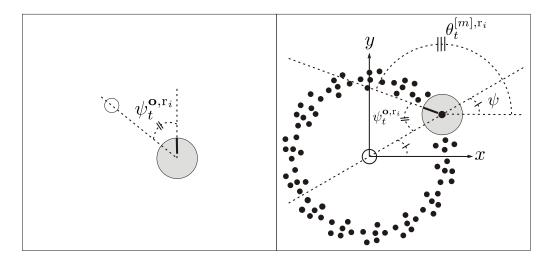
Figure 4.2: Computing the orientation of an  $m^{\text{th}}$  particle representing a robot pose hypothesis. On the left, bearing of the object with respect to the robot. On the right: relevant angles for the computation of the orientation component of the  $m^{\text{th}}$  particle as per (4.1).
