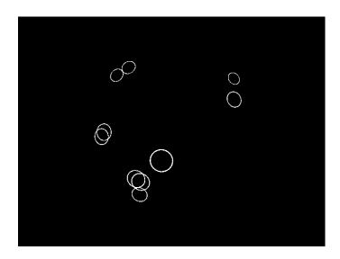
Figure 2.4: Binary edge image containing the projected tear-drop curves for a set of random 3D positions of a known-diameter sphere.
