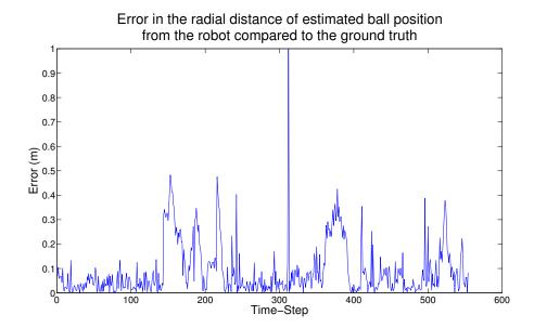
Figure 2.10: Error in the estimated radial distance of the ball position from the robot at each step of the PF iteration.
