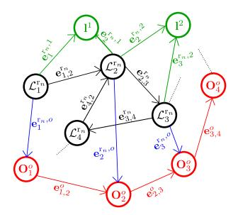
Figure 5.1: An example of the pose-graph representation of the O-MMLG depicting the robot  $\mathbf{r}_n$  in the team, the  $o^{\text{th}}$  object (moving landmark), static and known landmarks numbered  $\mathbf{l}^1$  and  $\mathbf{l}^2$  and the edges connecting all these nodes. The notations are as described in Section 5.3.2.
