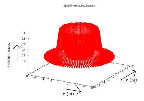
Figure 4.1: Typical spatial probability density function from which particles are drawn, after a decision to reset MCL.
