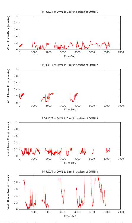
Figure 5.9: PF-UCLT: robots' estimated position error plots for the 4 robots experiment.
