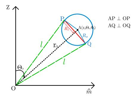
Figure 2.3: Cross-section of Figure 2.2 along the plane perpendicular to X-Y plane and at an azimuth of  $\Phi_0$ .  $\hat{m}$  is the vector along the azimuth of  $\Phi_0$  on the reference plane of the world frame in Figure 2.2.
