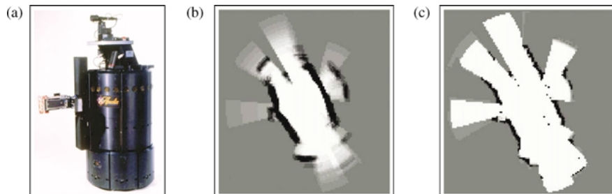
Figure 5. (a) The RWI B21 robot used in our experiments. This robot is equipped with a cyclic array of 24 Polaroid sonar sensors. (b) Comparison of conventional occupancy grid mapping with (c) our approach using forward models. The open doors are only visible in (c). However, several small obstacles are shown in (c) that stem from a person walking by the robot during data collection. Each grid consists of 114 by 120 grid with 10 centimeter resolution.
