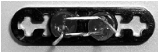
Figure 12-31. LEDs connected in parallel
