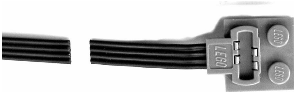
Figure 11-32. Cut Power Functions connector off the motor
