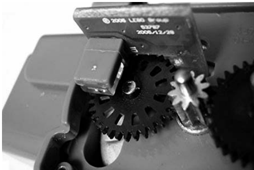
Figure 1-30. Close up of Rotation Sensor
