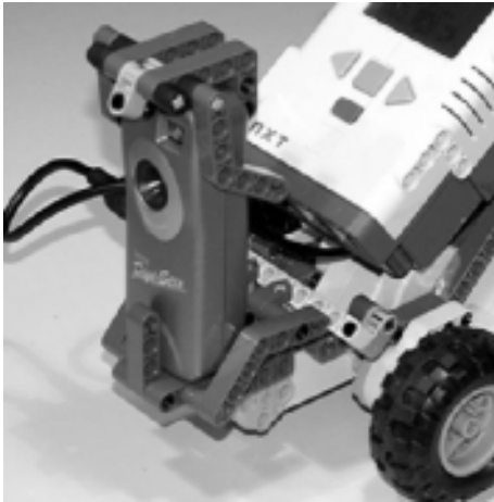
Figure 14-32. Inexpensive digital camera fitted to the vehicle
