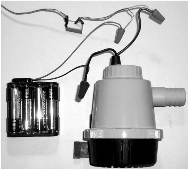
Figure 12-17. Relay control of a 12V bilge pump
