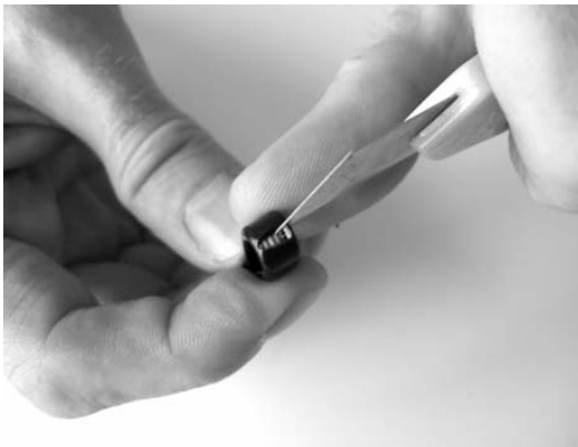
Figure 3-16. Cut cable method step 1: cut the jacket
