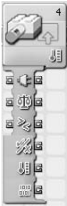
Figure 5-10. Legacy Temperature block
