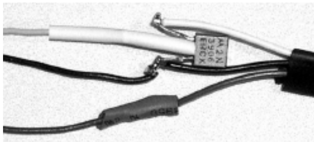
Figure 8-18. Transistor buffer for the GP2D12 interface
