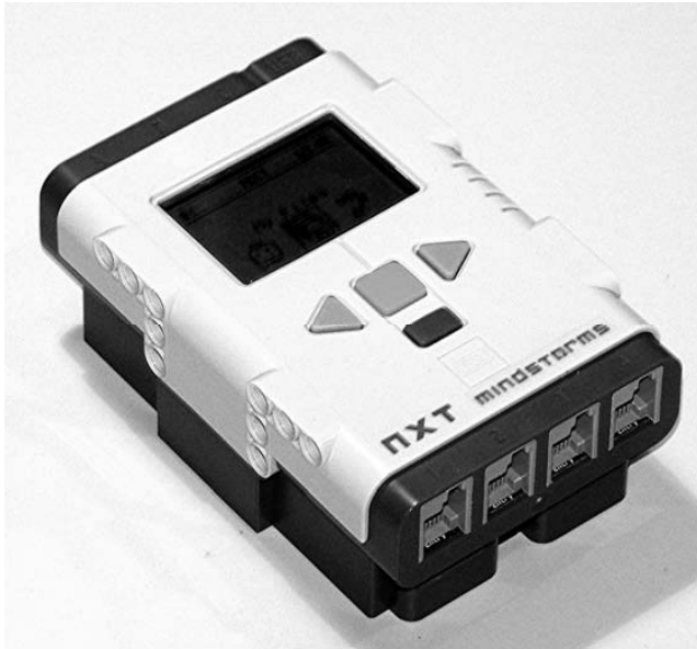
Figure 1-4. The NXT programmable brick
