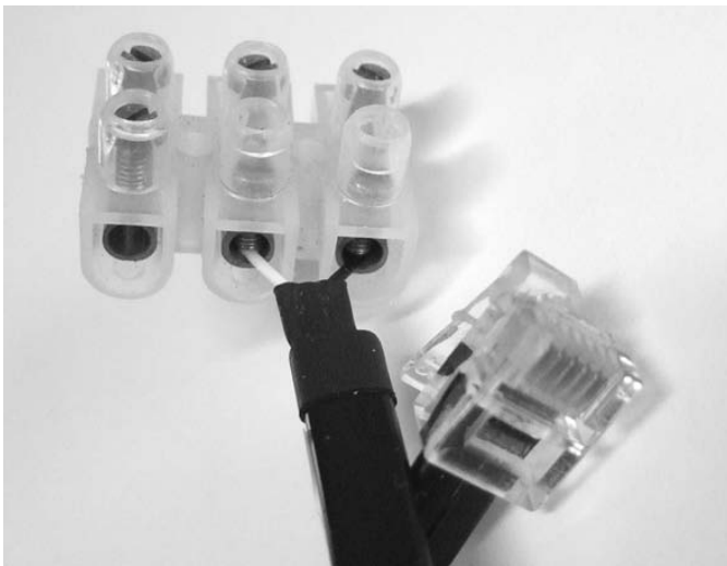
Figure 3-23. Screw terminal cable for passive sensor prototyping
