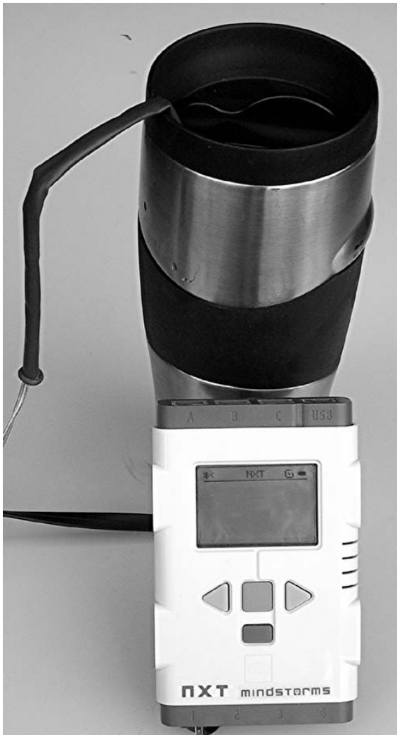
Figure 5-23. Measuring the temperature of ice water
