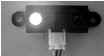
Figure 8-15. Infrared beam as seen with a digital camera
