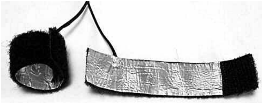
Figure 14-43. Completed finger electrodes
