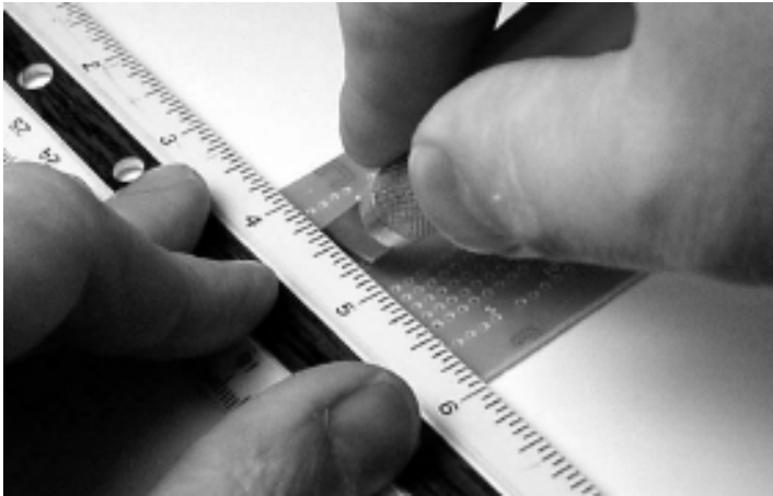
Figure A-8. Scoring the PC board
