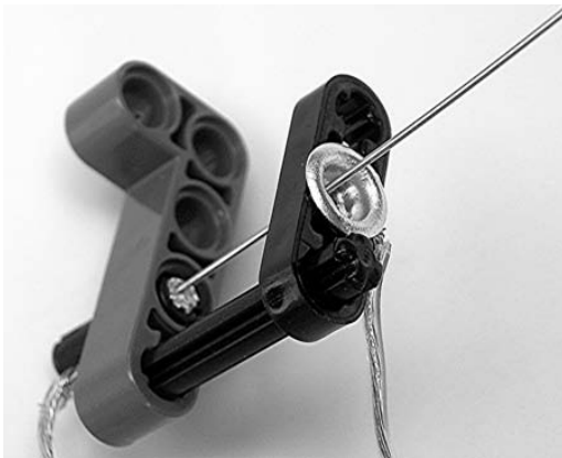
Figure 4-17. Finished antenna sensor
