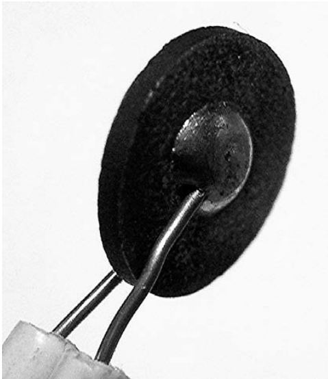
Figure 5-13. Semiconducting pellet inside a thermistor
