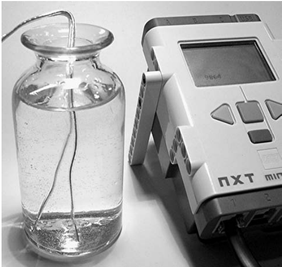
Figure 5-7. Measuring the salinity of water
