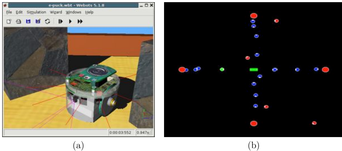
Figure 2.2: (a) The e-puck robot module in a Webots simulation. (b) twodeepuck simulation screenshot (small circles represent agents).
