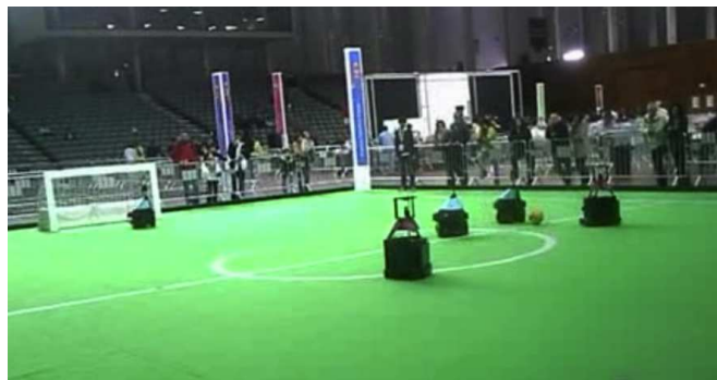
Figure 3.1: A typical in-game situation in RoboCup Middle-Size League Robotic Soccer, showing cooperation between two robots.
