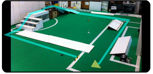
Fig. 4. Scenario used for experimental results. The indicated line represents the trajectory travelled by RAPOSA-NG during the experiment. The starting point is marked with black/yellow strips, and the path proceeds clockwise (with respect to the top view).
